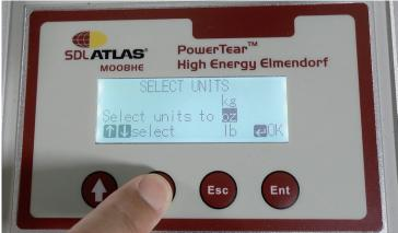
cN, N, g, k, oz and lbs. Results are displayed on an integral 16 character LCD screen at the end of each test. The display also shows the sample number and
